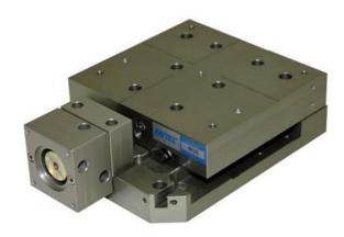
The Q-Max precision positioning stage series from NUTEC developed for maximum stiffness and high resolution. A short stroke translation stage capable of precise positioning in either vertical or horizontal orientations, while maintaining extremely tight trajectory control.
